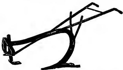
FIG. 70. Subsoiler that loosens the subsoil by breaking through.
